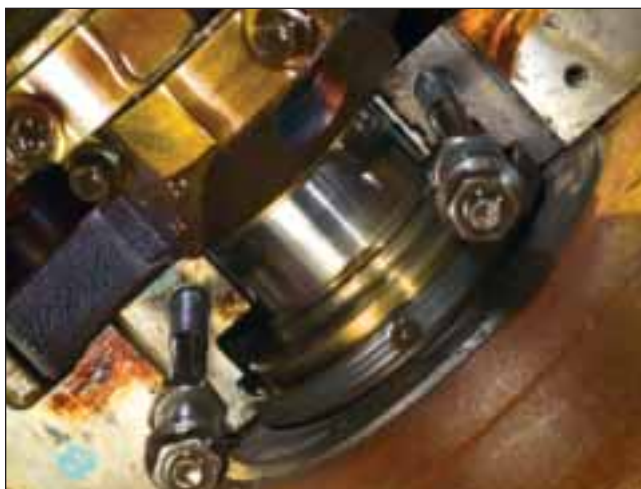
A closeup view of the rear main crankshaft journal. No visible wear detected.
